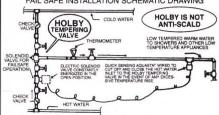
PIPING DIAGRAM SHOWING THE USE AND APPLICATION OF A CONSTANTLY ENERGIZED ELECTRIC SOLENOID VALVE, WIRED TOGETHER WITH A QUICK ACTING AND SENSING IMMERSION AQUASTAT (MERCURY TYPE PREFERRED FOR VISUAL INSPECTION.)
