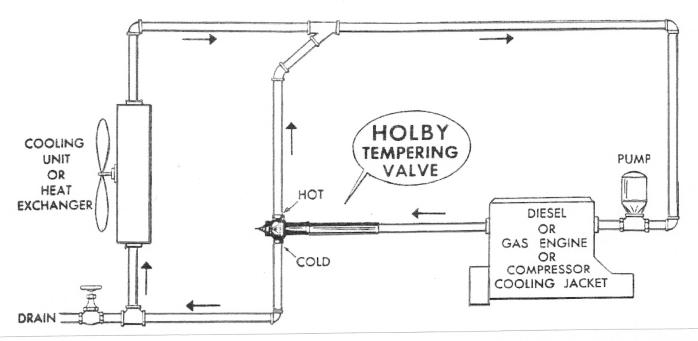
When temperature of cooling fluid from engine cooling jacket is within the normal range, the flow is passed through the "HOT" port of the HOLBY VALVE and then back to the engine cooling jacket.
